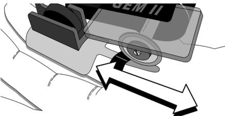
7. Use GEM II ring spreader pliers or forceps to remove ring.
