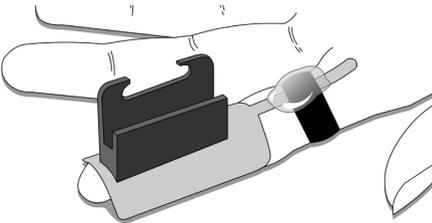
5. Move GEM II back and forth along guide block so that cutting disc traverses the entire width of the ring. A sudden increase in rotation speed indicates ring has been cut through.
