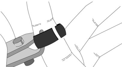
2. Apply a generous quantity of water based gel to ring surface.
